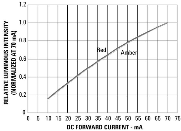
Figure 3. Relative Luminous Intensity vs. Forward Current
