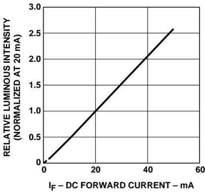
Figure 3. Relative Luminous Intensity vs. Forward Current.
