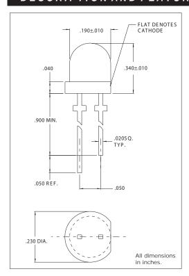
The Ultrabright HLMP3X50 series are direct pin for pin replacements for Hewlett Packard's HLMP3X50 series. These LED lamps provide a very narrow viewing angle in a clear tinted non-diffused package and are excellent for small area backlighting. A pale tint aids in identification. The High Efficiency Red and Yellow lamps are produced with GaAsP/GaP and the High Efficiency Green lamp is produced with GaP/GaP. All feature an 80 mcd minimum luminous intensity.
