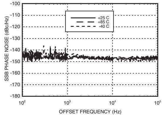
**Phase Noise Floor vs Offset Frequency
