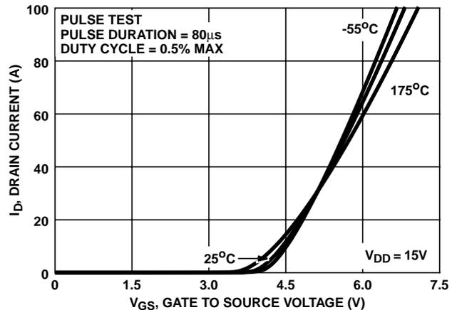
FIGURE 8. TRANSFER CHARACTERISTICS
