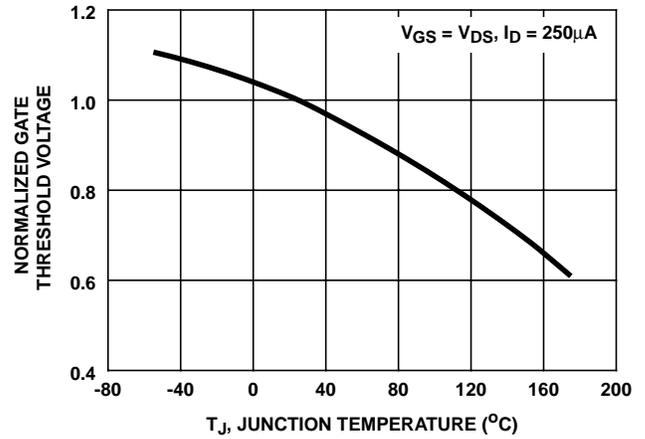
FIGURE 10. NORMALIZED GATE THRESHOLD VOLTAGE vs JUNCTION TEMPERATURE
