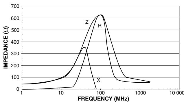
**TYPICAL CURVES** (Frequency Characteristics of R, X, and Z)ILHB-1812 1300  $\Omega$
