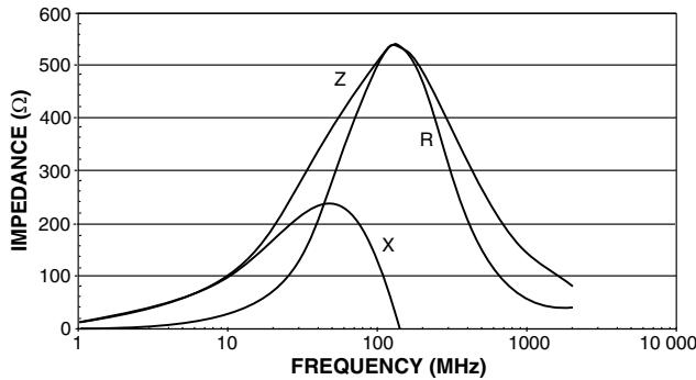
**TYPICAL CURVES** (Frequency Characteristics of R, X, and Z)
