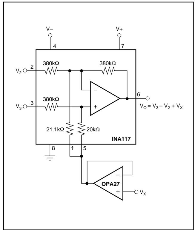
FIGURE 11. Summing V<sub>X</sub> in Output.
