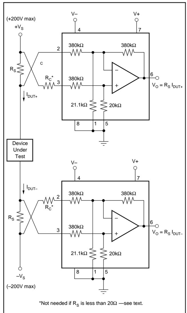
FIGURE 4. Measuring Supply Currents of Device Under Test.
