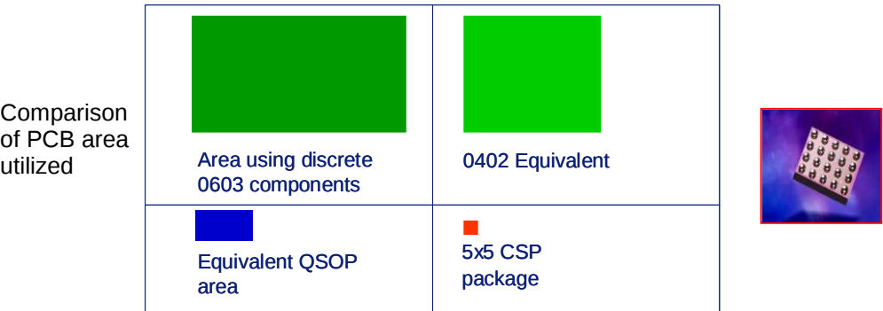
Fig 1. PCB area comparison of different package type for a 10-channel filter
