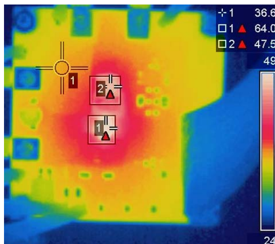
Figure 21: Thermal Image at V_{IN} = 12V , I_{OUT} = 6A (IR3473: 64^\circ C , Inductor: 48^\circ C , PCB: 37^\circ C )
