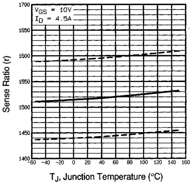
Fig 15. Typical HEXSense Ratio Vs. Junction Temperature
