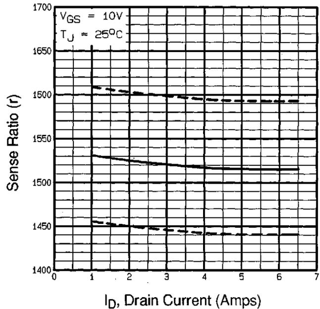
Fig 16. Typical HEXSense Ratio Vs. Drain Current
