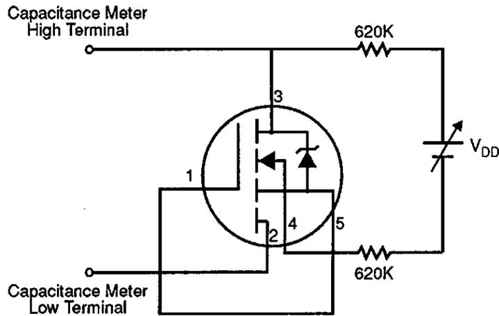
Fig 19. HEXSense Sensing Cell Output Capacitance Test Circuit
