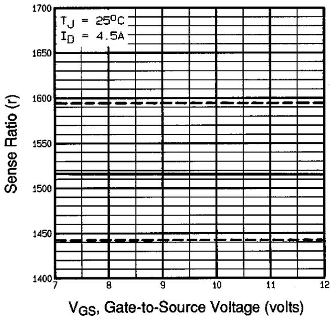
Fig 17. Typical HEXSense Ratio Vs. Gate Voltage
