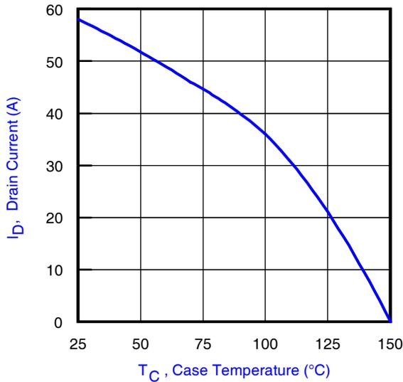
**Fig 12.** Maximum Drain Current vs. Case Temperature
