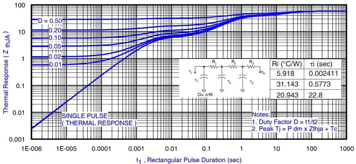
**Fig 3. Maximum Effective Transient Thermal Impedance, Junction-to-Ambient ③**
