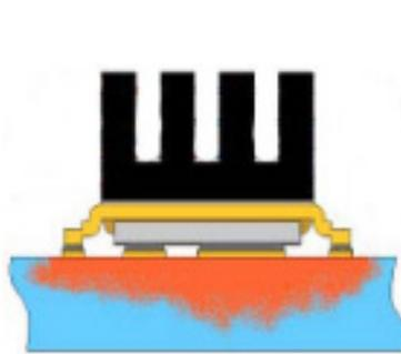
⑥ Mounted to a PCB with small clip heatsink (still air)
