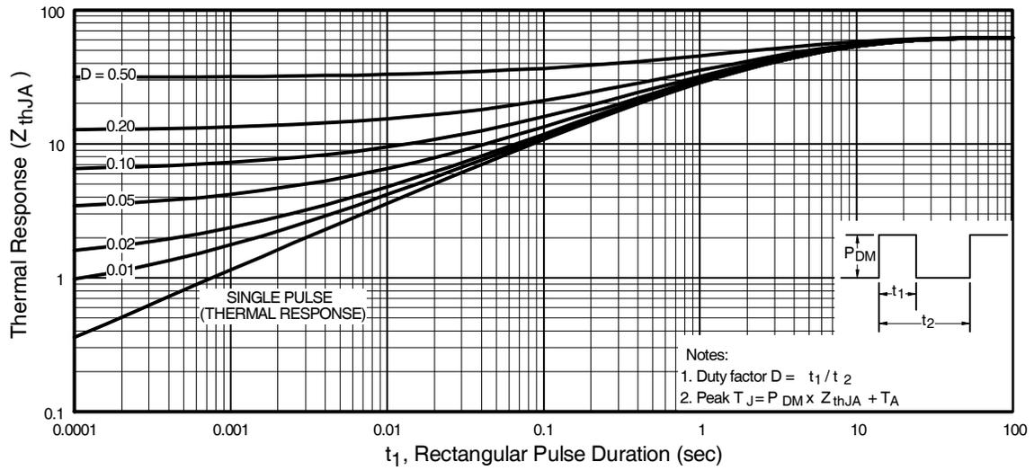
**Fig 10.** Maximum Effective Transient Thermal Impedance, Junction-to-Ambient
