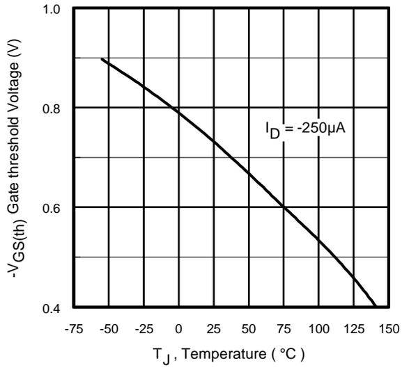
**Fig 15.** Typical V<sub>gs(th)</sub> Vs. Junction Temperature
