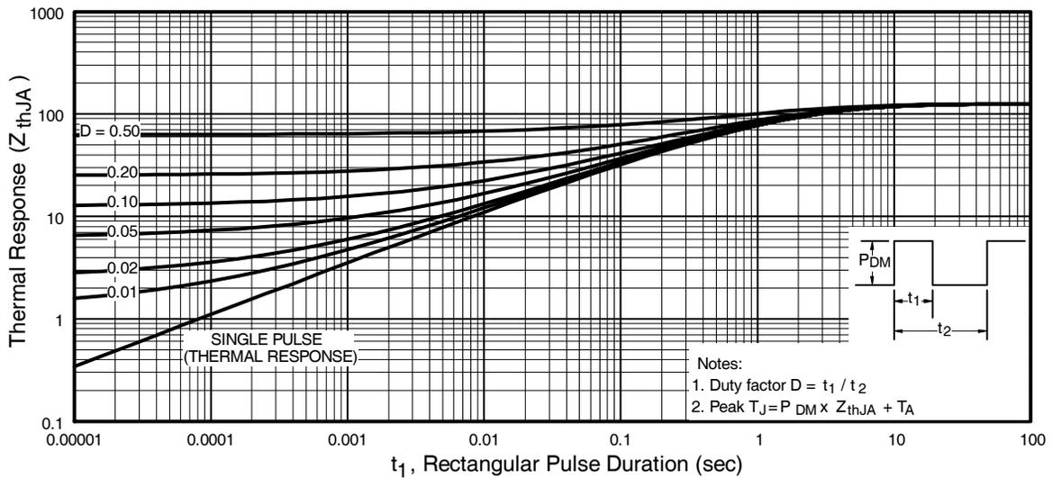
**Fig 10.** Typical Effective Transient Thermal Impedance, Junction-to-Ambient
