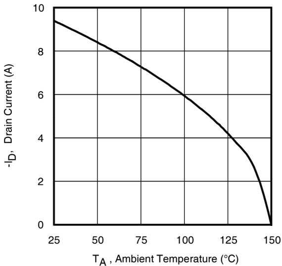
**Fig 9.** Maximum Drain Current vs. Ambient Temperature
