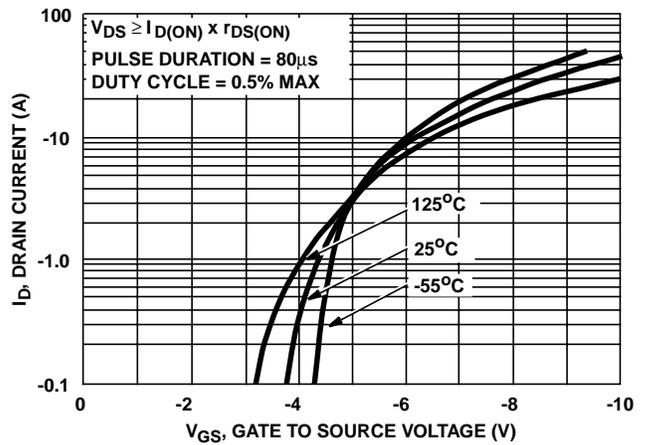
FIGURE 7. TRANSFER CHARACTERISTICS
