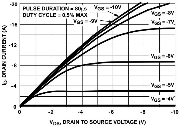
FIGURE 6. SATURATION CHARACTERISTICS
