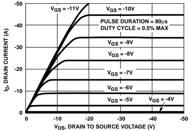
FIGURE 5. OUTPUT CHARACTERISTICS
