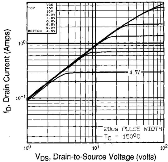
**Fig. 2 - Typical Output Characteristics,  $T_C = 150^\circ\text{C}$**
