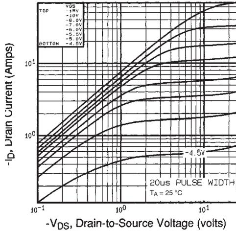
Fig. 1 - Typical Output Characteristics,  $T_A = 25\text{ °C}$
