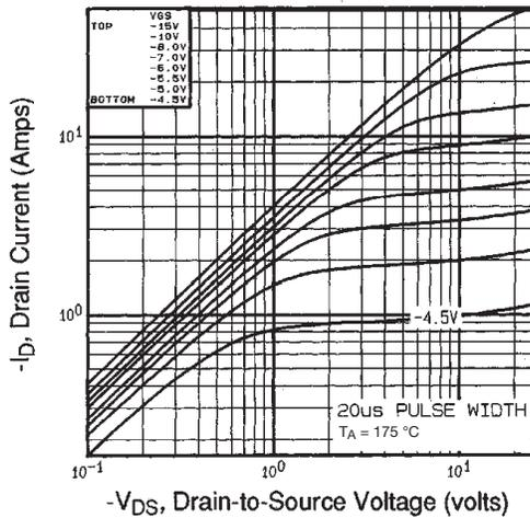
Fig. 2 - Typical Output Characteristics,  $T_A = 175\text{ °C}$
