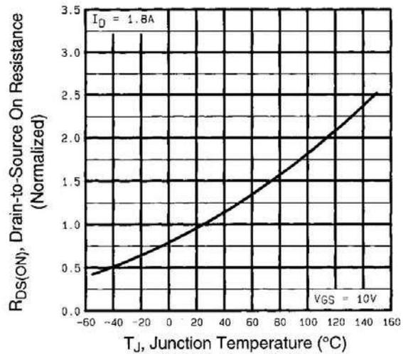
**Fig 4.** Normalized On-Resistance
