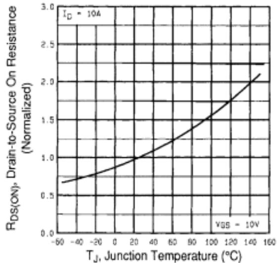
**Fig 4.** Normalized On-Resistance
