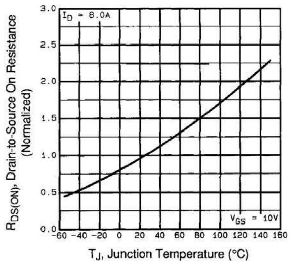
**Fig 4.** Normalized On-Resistance
