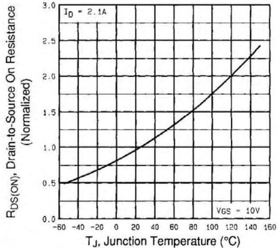
**Fig 4.** Normalized On-Resistance
