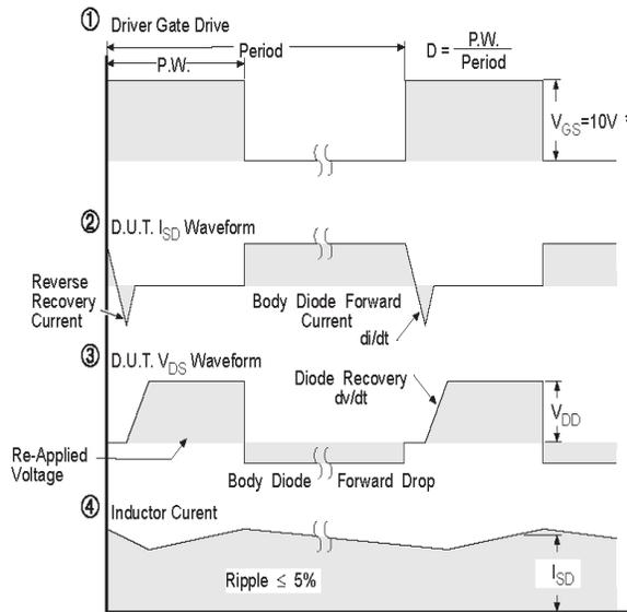
\*  $V_{GS} = 5V$  for Logic Level Devices
