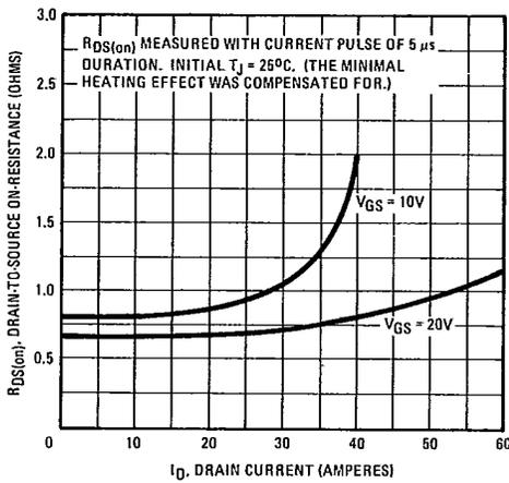
Fig. 12 - Typical On-Resistance Vs. Drain Current
