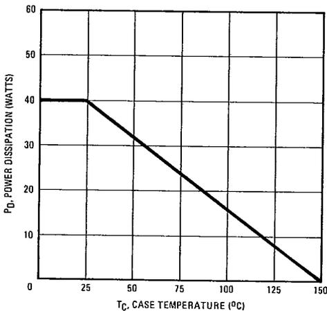
Fig. 14 - Power Vs. Temperature Derating Curve
