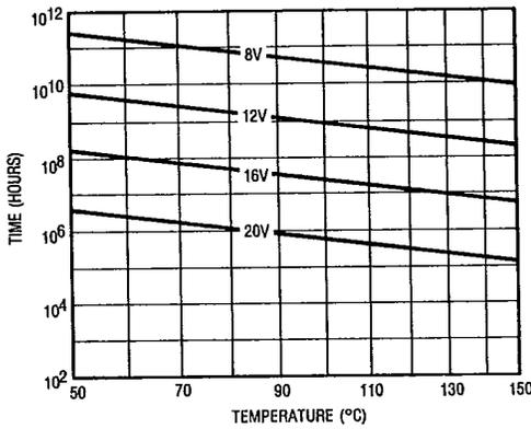
\*Fig. 19 — Typical Time to Accumulated 1% Failure
