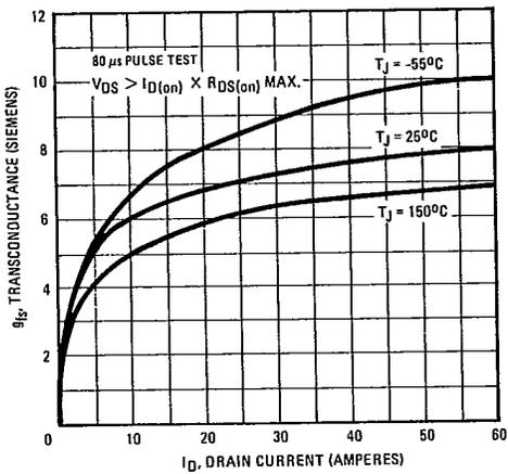
Fig. 6 – Typical Transconductance Vs. Drain Current
