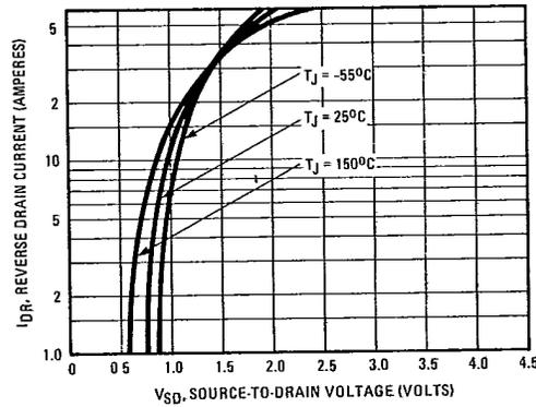
Fig. 7 – Typical Source-Drain Diode Forward Voltage
