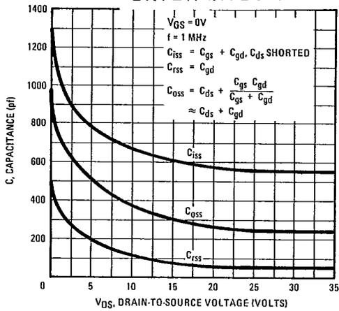
Fig. 10 - Typical Capacitance Vs. Drain-to-Source Voltage
