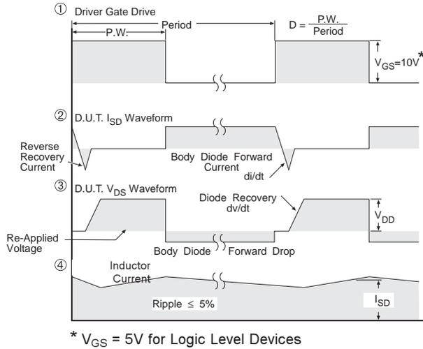
**Fig 16. Peak Diode Recovery  $dv/dt$  Test Circuit for P-Channel HEXFET<sup>®</sup> Power MOSFETs**
