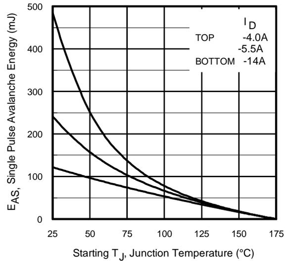
**Fig 13.** Maximum Avalanche Energy Vs. Drain Current
