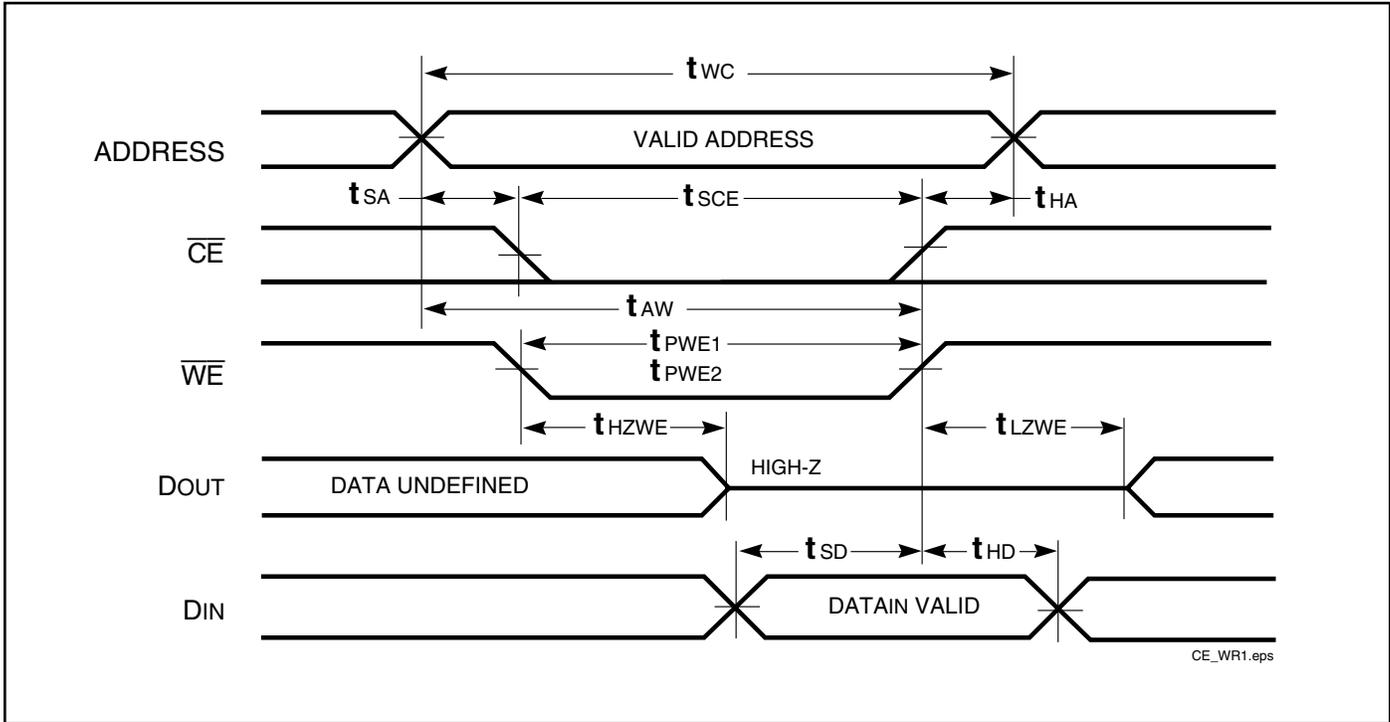
**WRITE CYCLE NO. 2**<sup>(1,2)</sup> ( $\overline{WE}$  Controlled:  $\overline{OE}$  is HIGH During Write Cycle)
