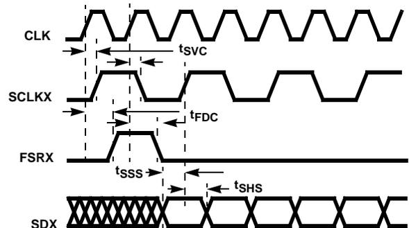
FIGURE 20. SERIAL INTERFACE RELATIVE TIMING
