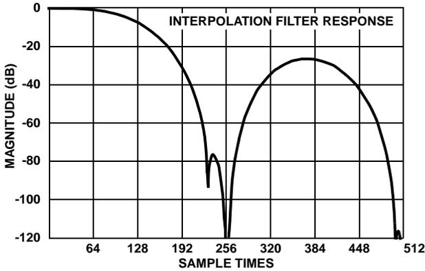
FIGURE 13B. INTERPOLATION FILTER IMPULSE RESPONSE
