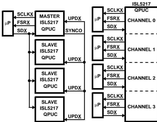
FIGURE 3. MULTIPLE CONFIGURATIONS
