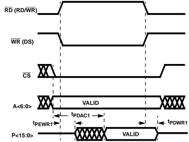
FIGURE 28. MICROPROCESSOR READ TIMING (RDMODE = 1)
