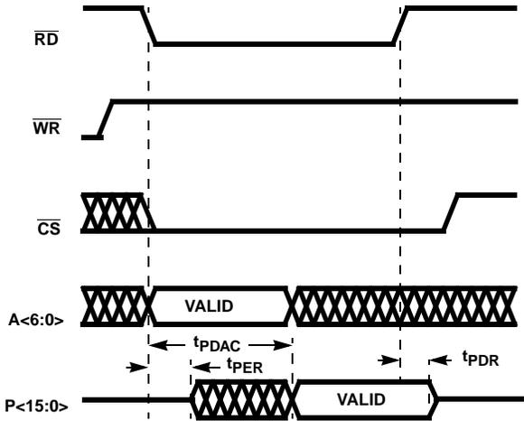
FIGURE 27. MICROPROCESSOR READ TIMING (RDMODE = 0)
