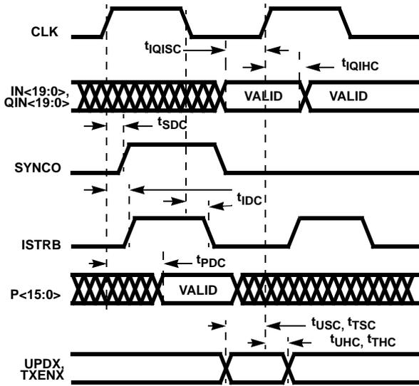
FIGURE 21. INPUT/OUTPUT TIMING
