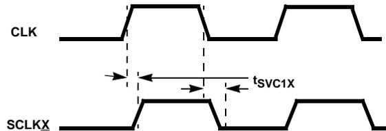
FIGURE 24. SCLKX OUTPUT TIMING IN 1X MODE
