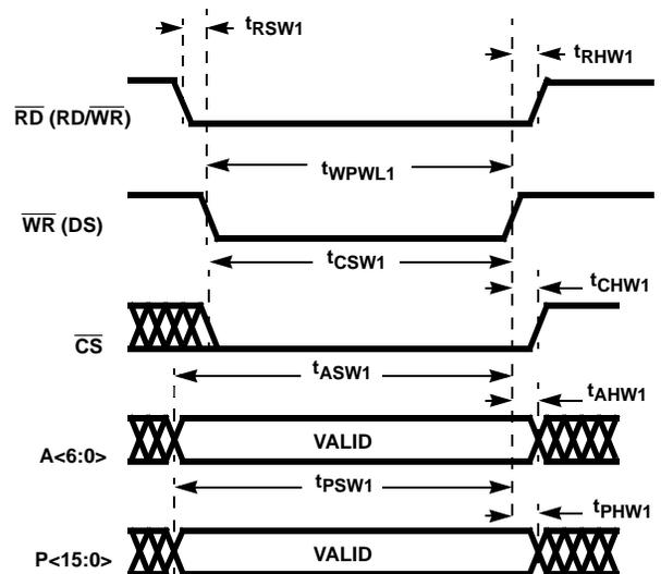
FIGURE 26. MICROPROCESSOR WRITE TIMING (RDmode = 1)
