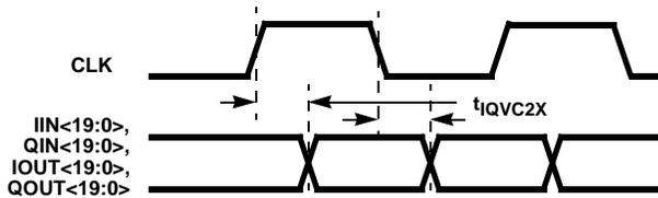
FIGURE 23. MUXED IQ AT 2X OUTPUT TIMING
