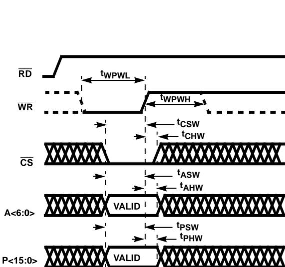
FIGURE 25. MICROPROCESSOR WRITE TIMING (RDmode = 0)
