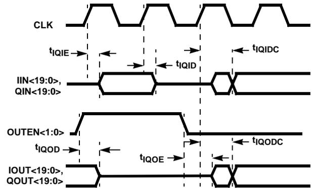
FIGURE 22. ENABLE/DISABLE TIMING
