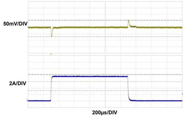
FIGURE 9. 1.2V<sub>OUT</sub> TRANSIENT RESPONSE
