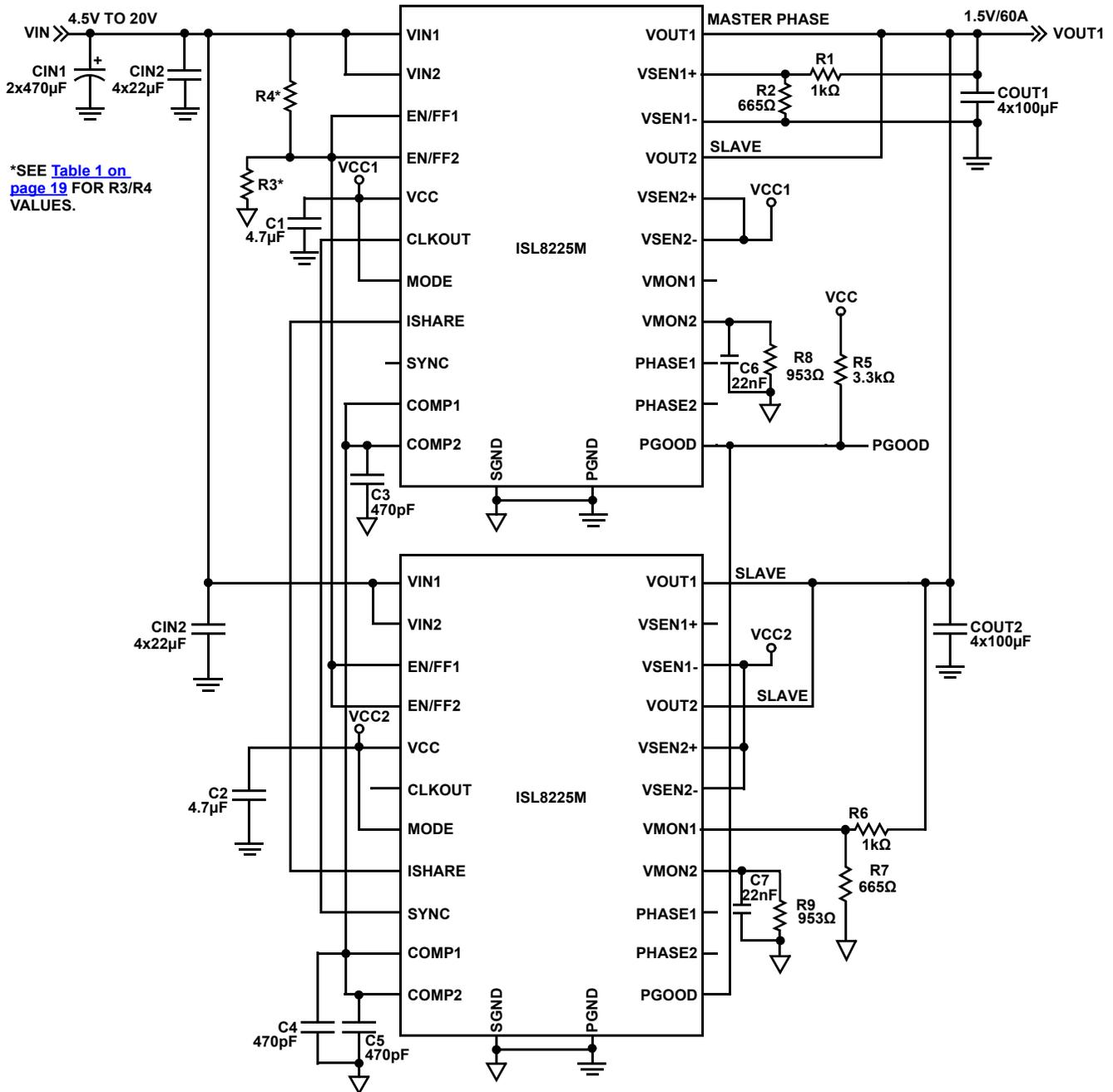
FIGURE 24. 4-PHASE PARALLELED AT 1.5V/60A WITH 90° INTERLEAVING
