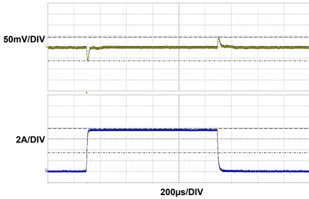
FIGURE 8. 1V<sub>OUT</sub> TRANSIENT RESPONSE
