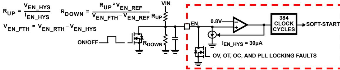
FIGURE 28. SIMPLIFIED ENABLE AND VOLTAGE FEED-FORWARD CIRCUIT
