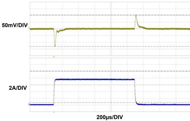
FIGURE 12. 2.5V<sub>OUT</sub> TRANSIENT RESPONSE
