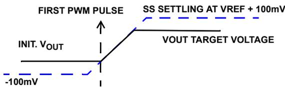
FIGURE 30. SOFT-START WITH  $V_{OUT} < \text{TARGET VOLTAGE}$
