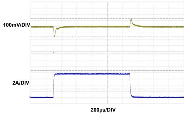
FIGURE 13. 3.3V<sub>OUT</sub> TRANSIENT RESPONSE
