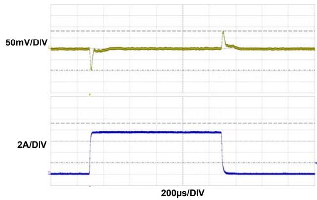
FIGURE 11. 1.8V<sub>OUT</sub> TRANSIENT RESPONSE
