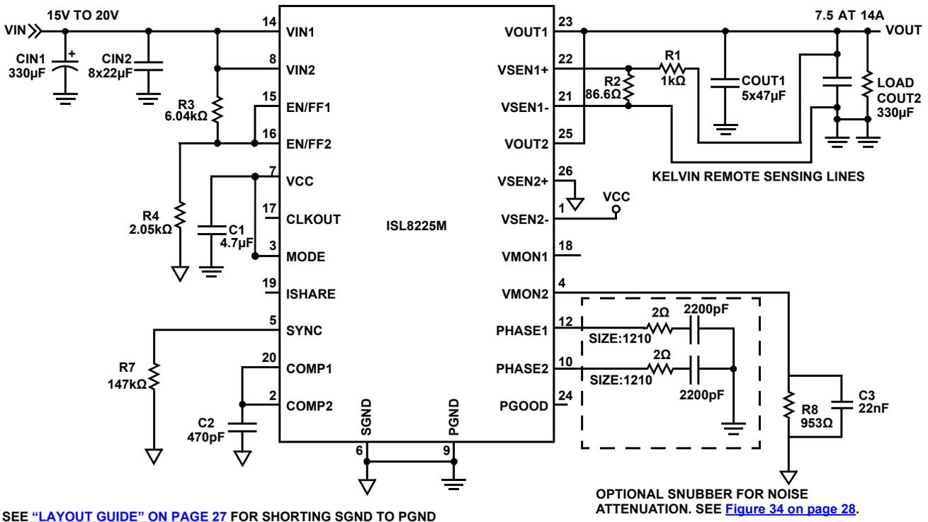
FIGURE 23. PARALLEL USE FOR SINGLE OUTPUT WITH 240° INTERLEAVING
