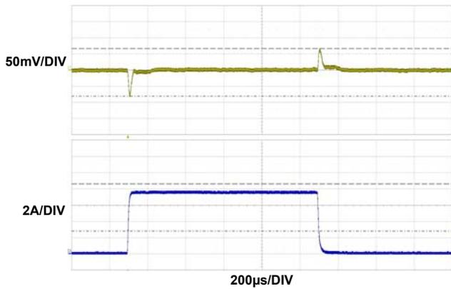
FIGURE 10. 1.5V<sub>OUT</sub> TRANSIENT RESPONSE
