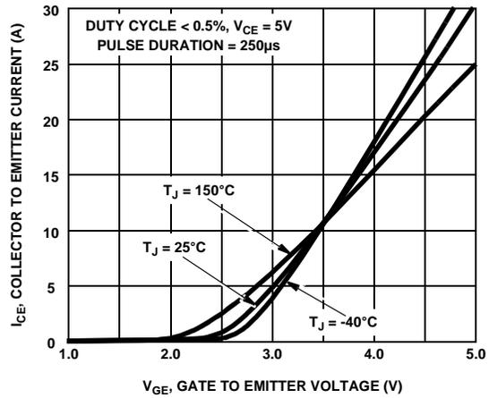
Figure 8. Transfer Characteristics
