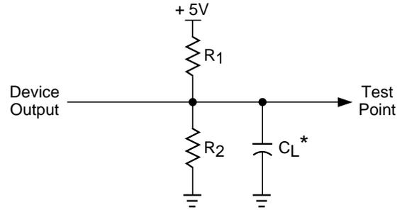
\*CL includes Test Fixture and Probe Capacitance.
