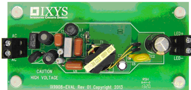
Figure 1. IX9908 Evaluation Board, Top View
