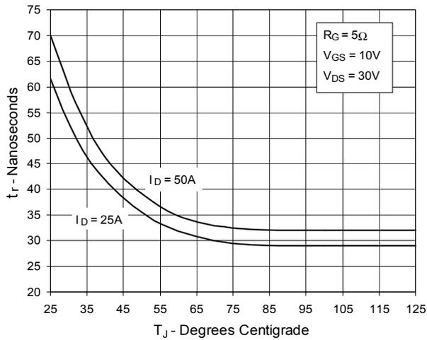
**Fig. 14. Resistive Turn-on Rise Time vs. Drain Current**
