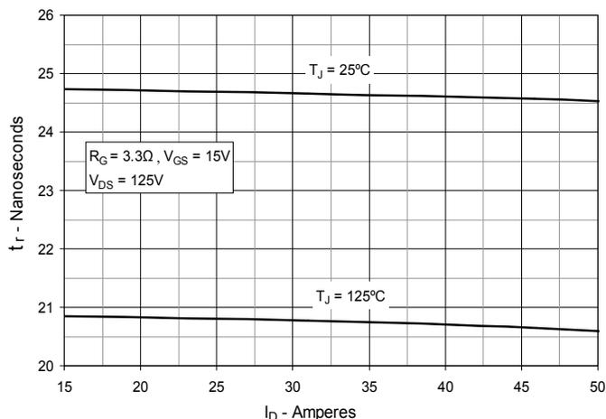
**Fig. 15. Resistive Turn-on
