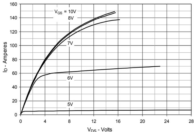
Fig. 3. Output Characteristics @  $T_J = 125^\circ\text{C}$
