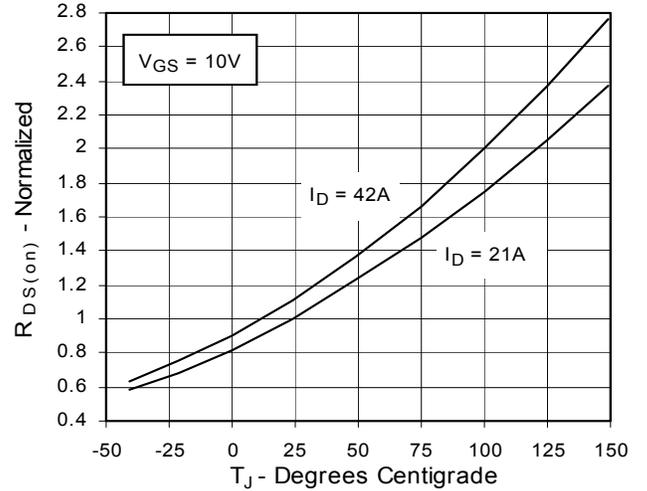
**Fig. 5.  $R_{DS(on)}$  Normalized to 0.5  $I_{D25}$  Value vs.  $I_D$**
