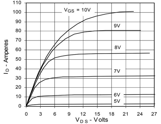
**Fig. 3. Output Characteristics**
