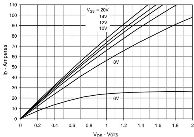
Fig. 2. Extended Output Characteristics @  $T_J = 25^\circ\text{C}$
