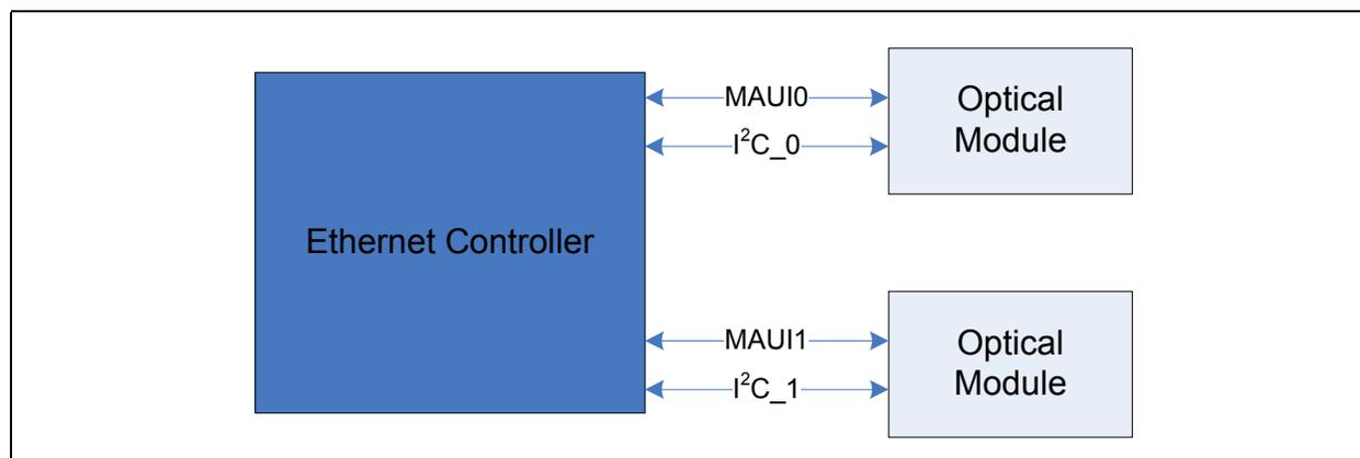
Figure 1.5. I<sup>2</sup>C Connection Example
