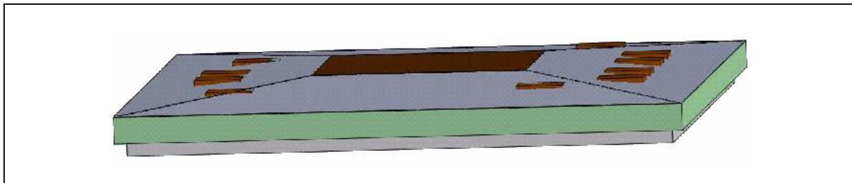
Figure 13-5. Die-Side Capacitors Exposed to Heat Sink Contact
