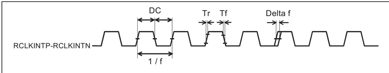
**Figure 11.14. External Clock Reference Timing**
