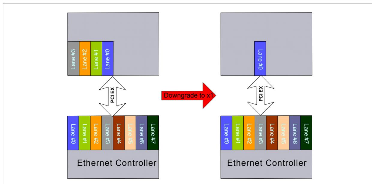
**Figure 3.5. Lane Downshift in an x4 Reversal Configuration**
