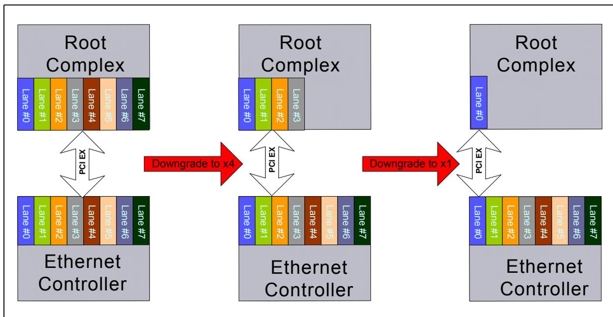
Figure 3.2. Lane Downshift in an x8 Configuration
