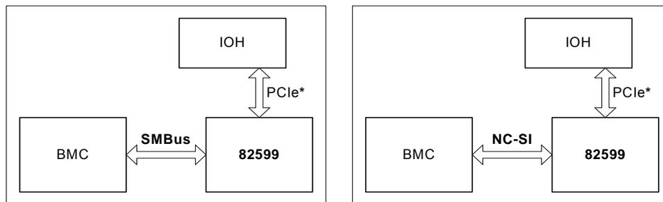
**Figure 10.1. the 82599 to BMC Connectivity Through SMBus Link or NC-SI Link**
