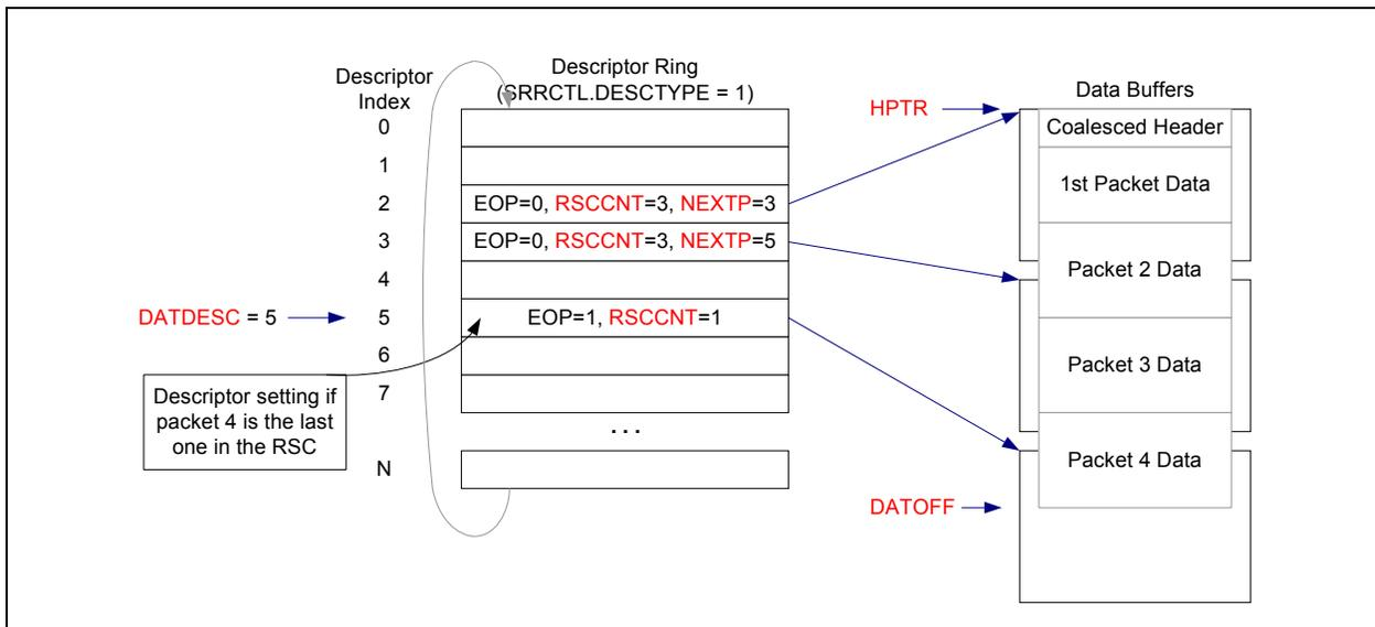
Figure 7.43. RSC Functionality (No Header Split)
