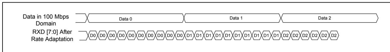
**Figure 3.19. Data Sampling in 100 Mb/s Mode**
