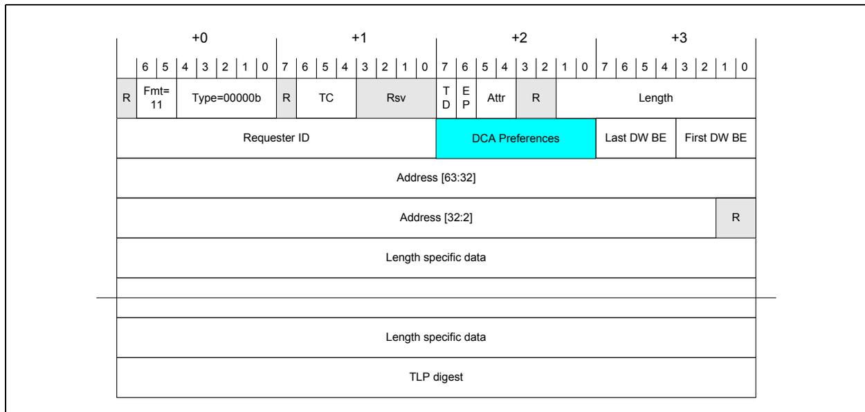
Figure 7.30. PCIe Message Format for DCA
