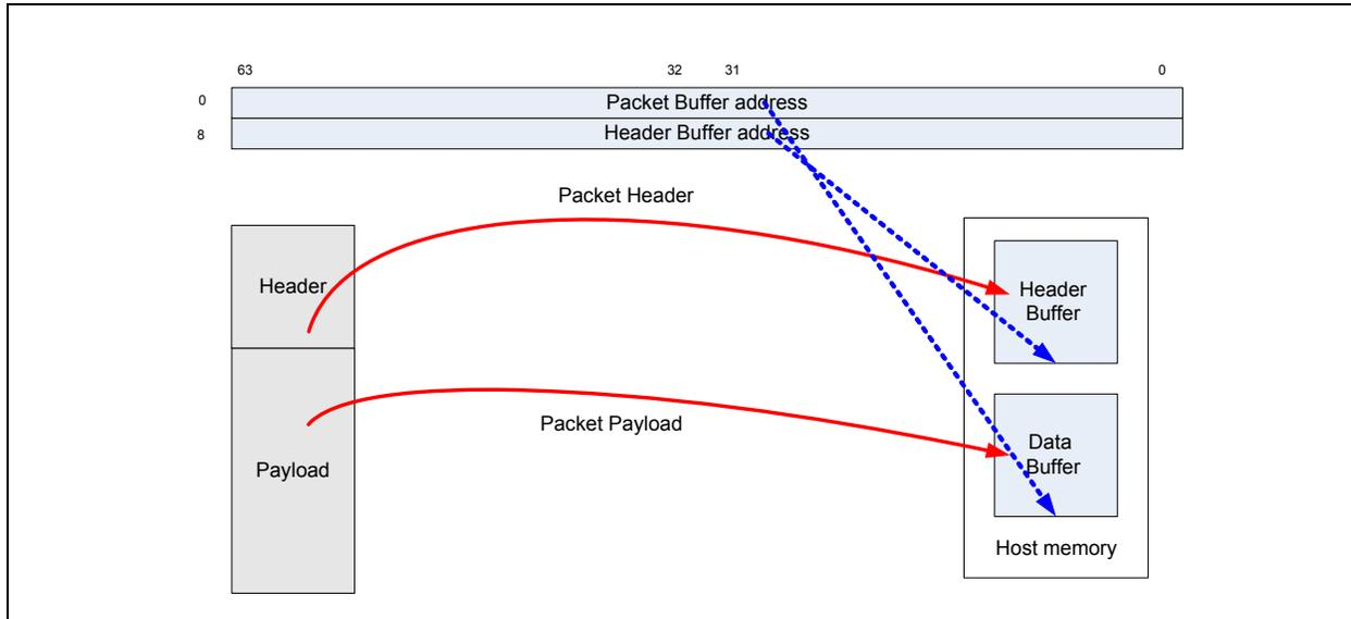
**Figure 7.13. Header Splitting Diagram**
