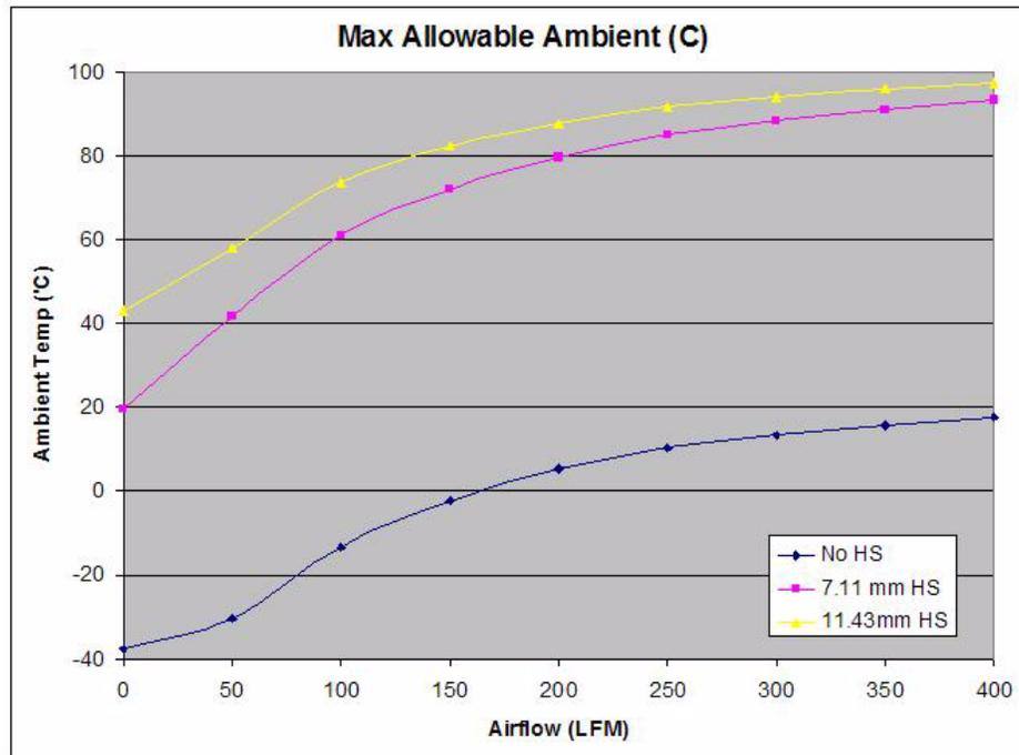
Figure 13-1. 82599 Max Allowable Ambient @ 8.82W (JEDEC Card)
