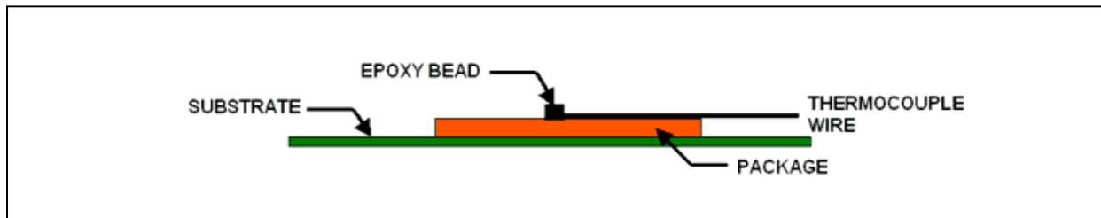
Figure 13-7. Technique for Measuring T<sub>case</sub> with 0° Angle Attachment, No Heatsinks
