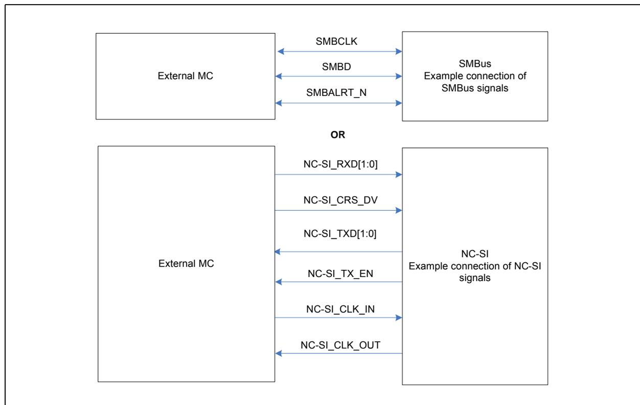
Figure 12-18. External MC Connections with NC-SI and SMBus
