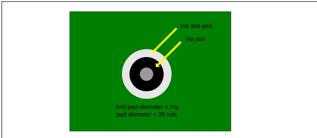
Figure 12-12. Increase Anti-Pad Diameter To Reduce Shunt Capacitance
