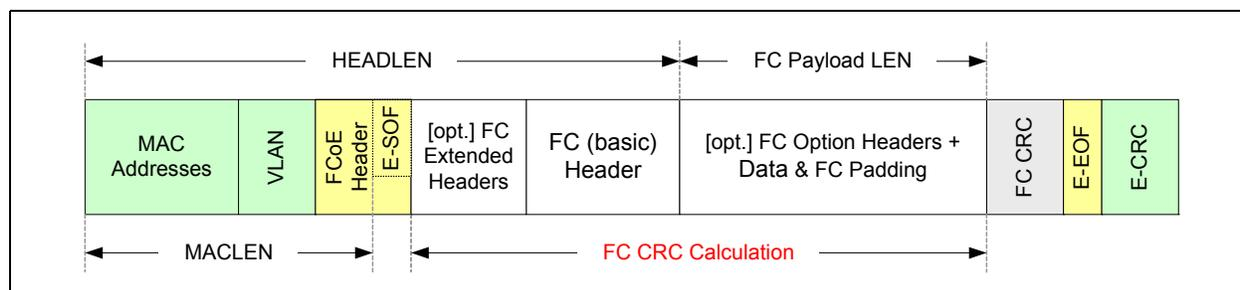
**Figure 7.48. FCoE Frame and Relevant Transmit Descriptor Parameters**
