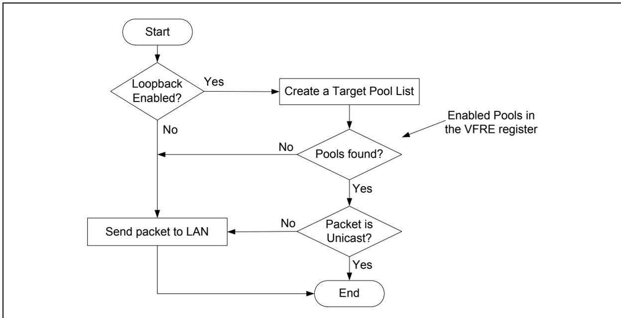
Figure 7.41. Tx Filtering
