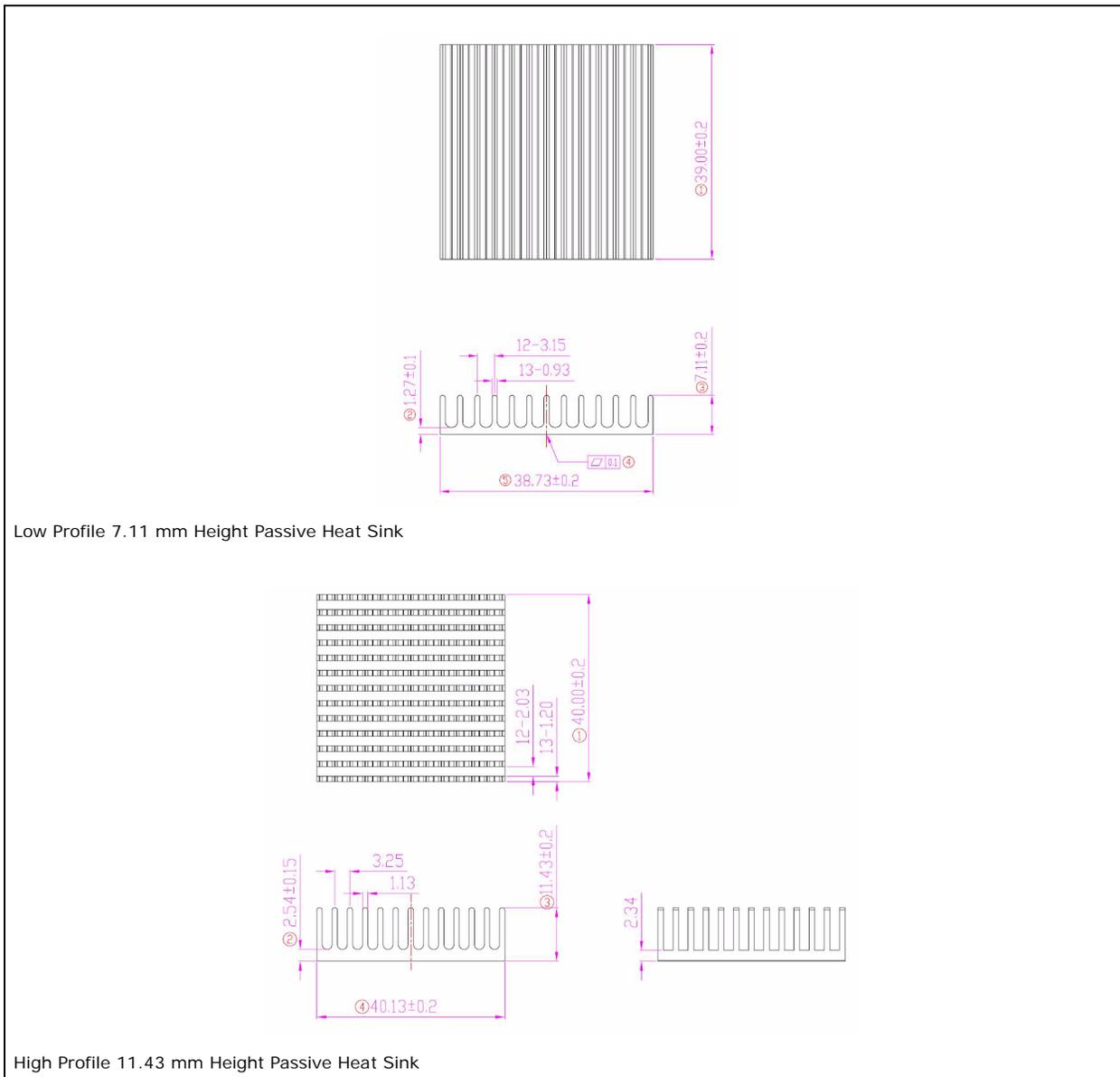
Figure 13-4. Extruded Heatsinks
