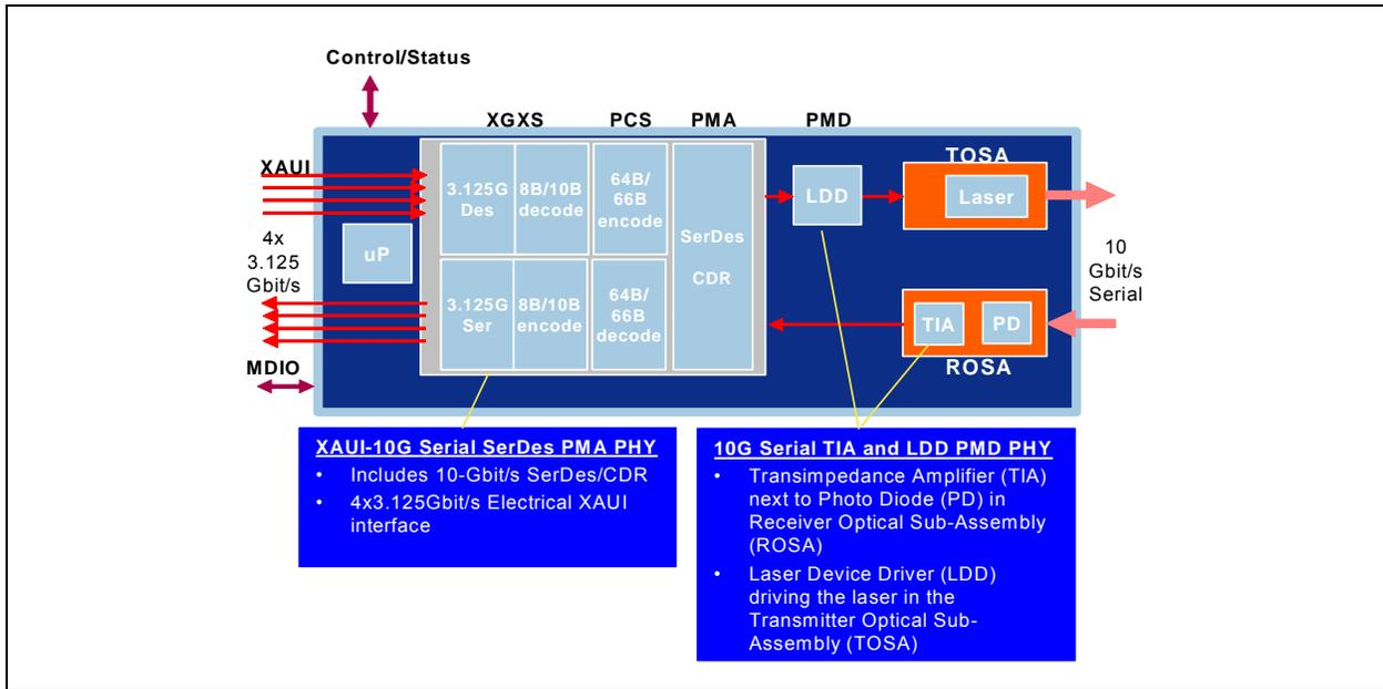
Figure 3.20. XENPAK, XPAK and X2 Transceiver Architecture
