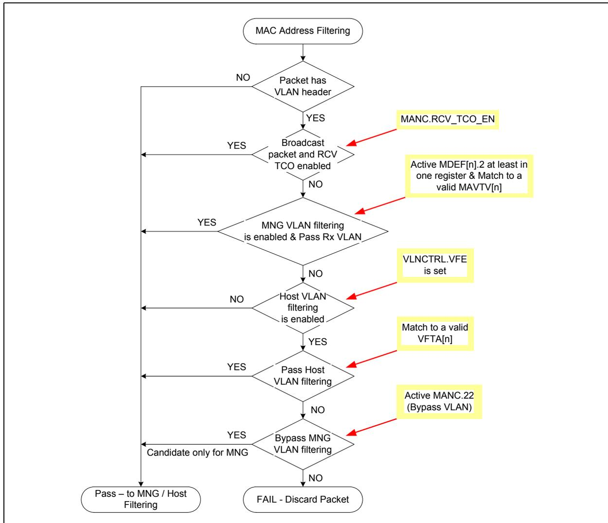
Figure 7.3. VLAN Filtering
