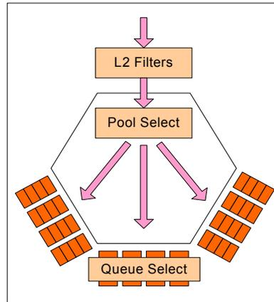
**Figure 7.1. Stages in Packet Filtering**
