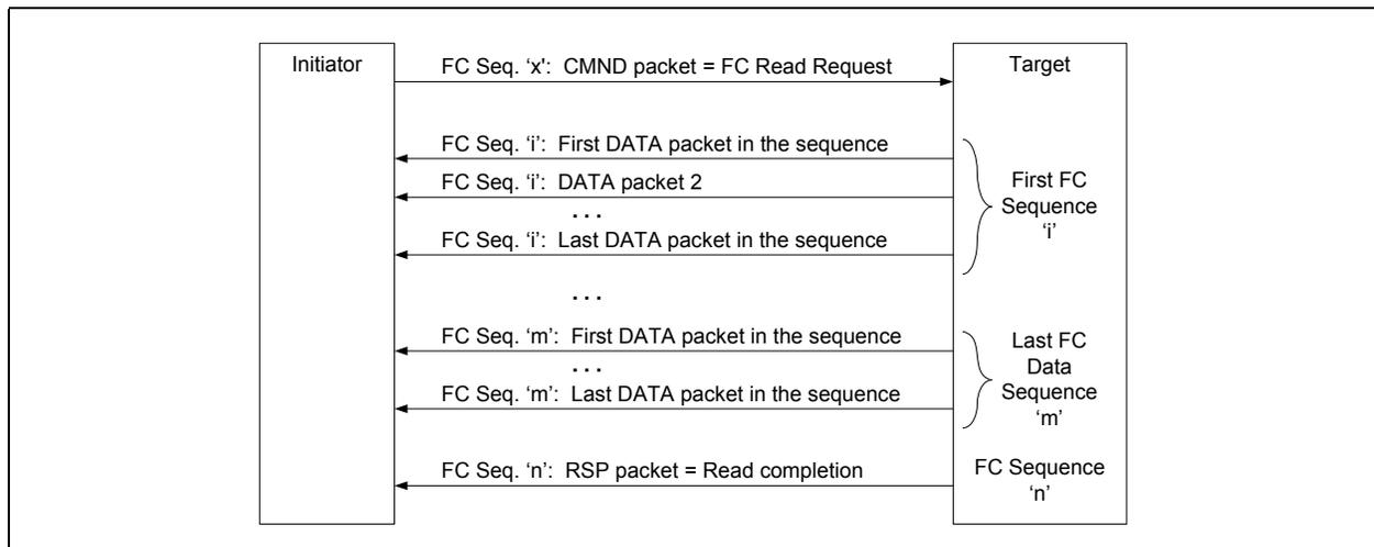
Figure 7.53. Example for FC Class 3 Read Exchange Flow
