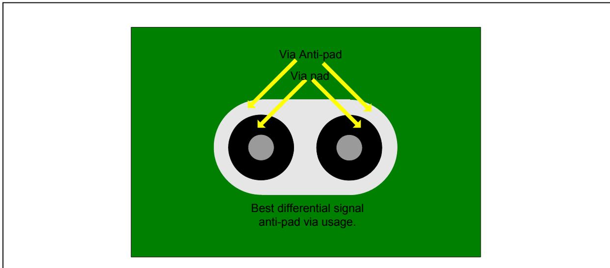
Figure 12-15. Best Differential Signals Via Anti-Pads
