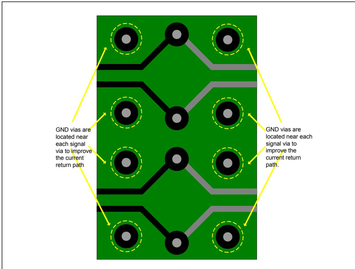
**Figure 12-9. Better Ground Vias for Signal Return Paths – Two Return Path Vias Per Signal Via (Less Reflection)**
