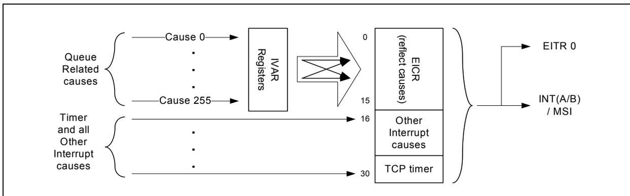
Figure 7.21. Cause Mapping in Legacy and MSI Modes
