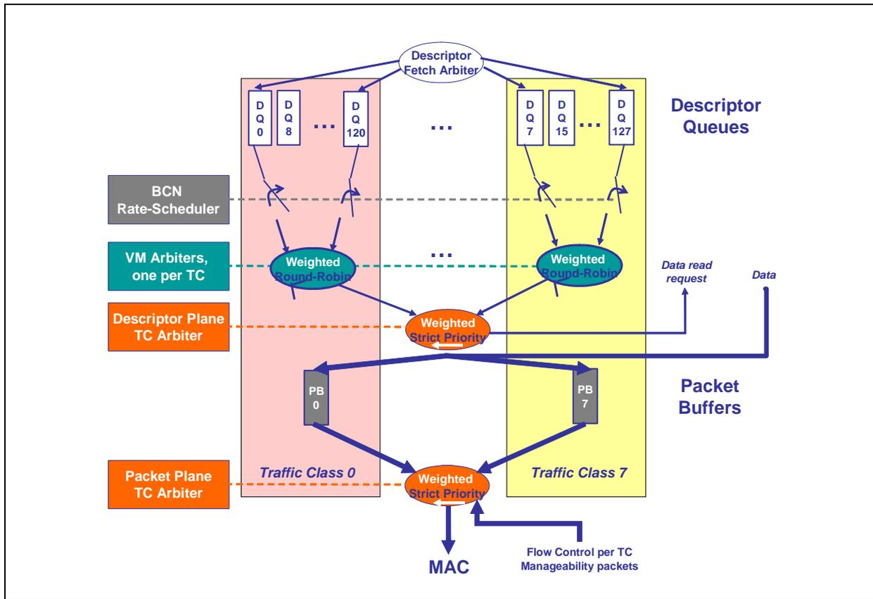
Figure 7.16. Transmit Architecture DCB-on/VT-on — Eight TCs Mode
