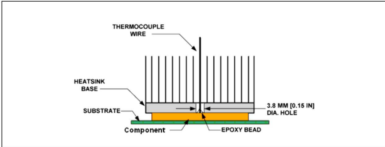
Figure 13-8. Technique for Measuring Tcase with 90° Angle Attachment
