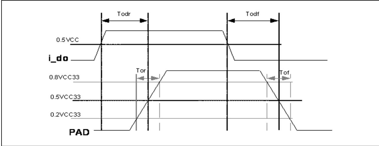
Figure 11.2. Digital 3.3V I/O Output Timing Diagram
