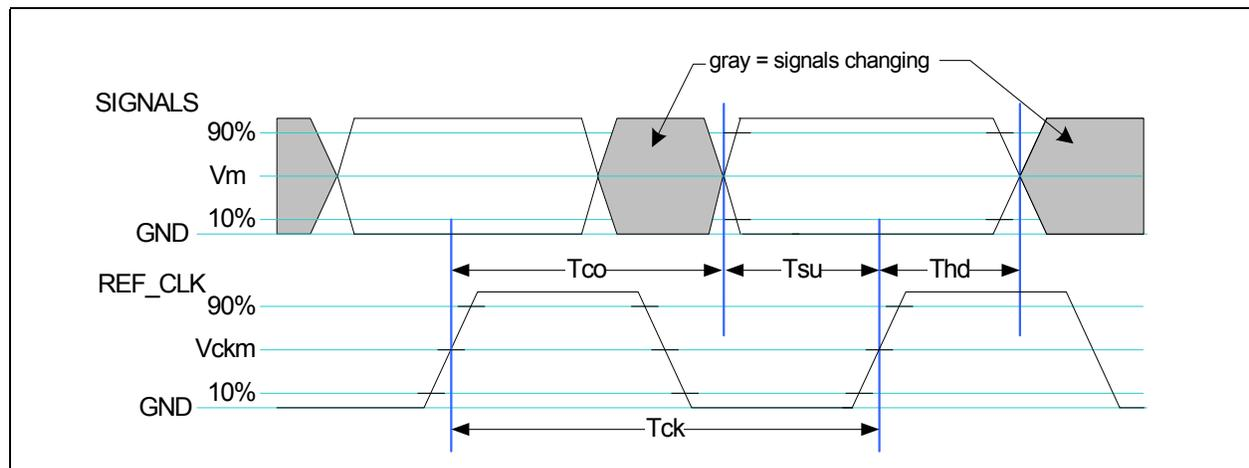
**Figure 11.7. NC-SI AC Timing Diagram**
