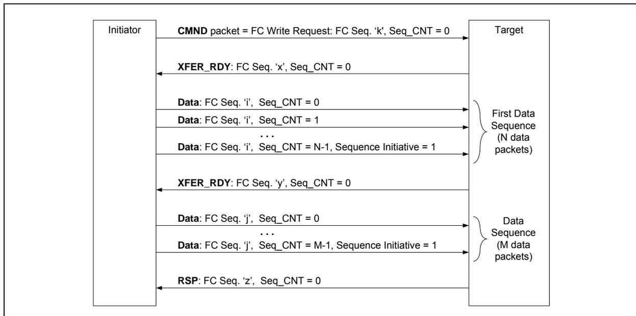
Figure 7.54. Example for FC Class 3 Write Exchange Flow
