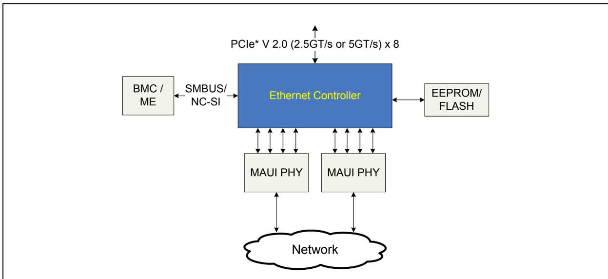
Figure 1.1. Typical Rack / Pedestal System Configuration
