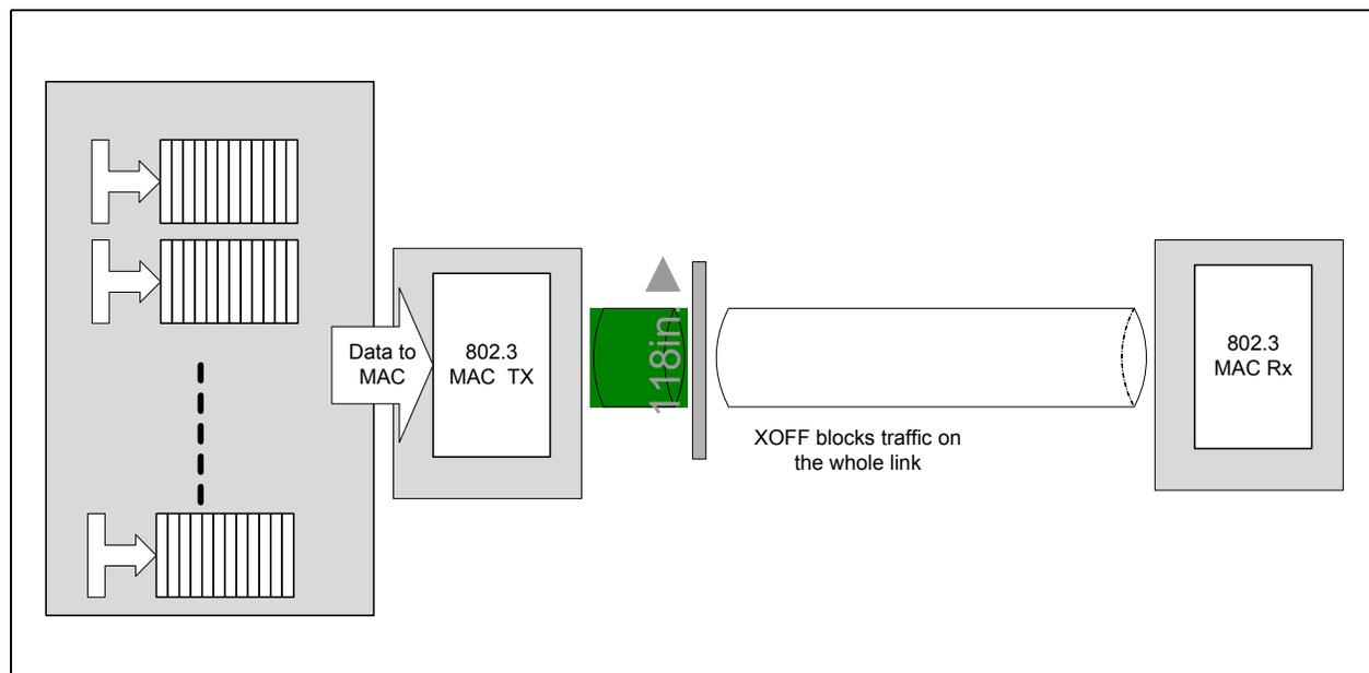
**Figure 3.25. 802.3X Link Flow Control (PAUSE)**
