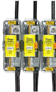
Bussmann power distribution fuse blocks are available preassembled into 1-, 2- and 3-pole versions. Individual blocks can be dovetailed together to achieve the desired number of poles. Use of covers requires ordering separately one cover for each pole.
