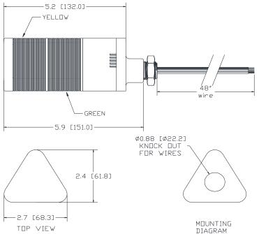
LED OPERATION: CONNECT STACK COLOR WIRE TO POWER AND BROWN WIRE TO POWER.
