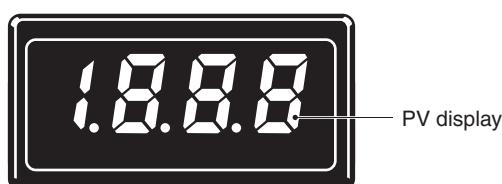
Select the decimal position with terminal 5, 6, or 7 on the rear panel.
