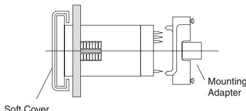
**Note:** Be sure to use the Water-resistive Soft Front Cover and mounting bracket together.
