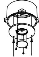
Secure the Filter assembly to the F-Mount adaptor using (3) 1/4" screws provided
