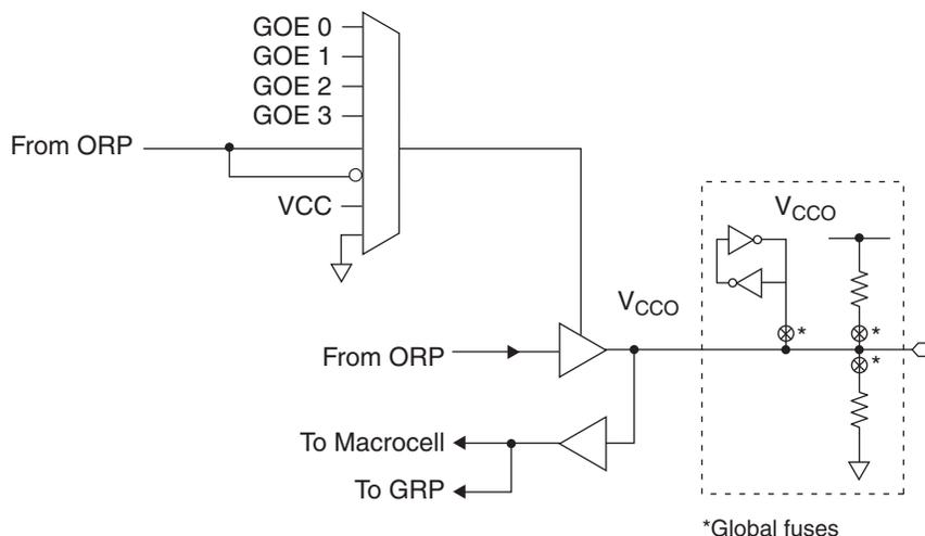
Each output supports a variety of output standards dependent on the  $V_{CC0}$  supplied to its I/O bank. Outputs can also be configured for open drain operation. Each input can be programmed to support a variety of standards, independent of the  $V_{CC0}$  supplied to its I/O bank. The I/O standards supported are:
