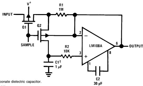
†Teflon, polyethylene or polycarbonate dielectric capacitor.
