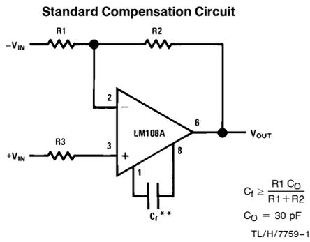
\*\*Bandwidth and slew rate are proportional to  $1/C_1$ .
