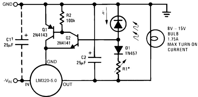
\*Lamp brightness increases until  $i_l = 5V/R1$  ( $i_l$  can be set as low as  $1 \mu A$ ).
