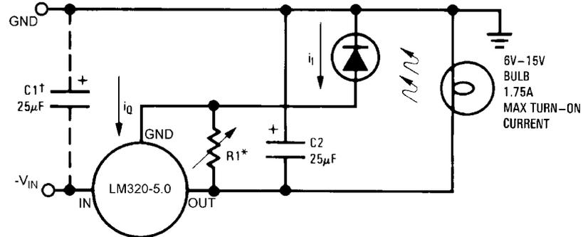
\*Lamp brightness increases until  $i_l = i_q (1 \text{ mA}) + 5V/R1$ .
