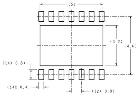
DIMENSIONS ARE IN MILLIMETERS
