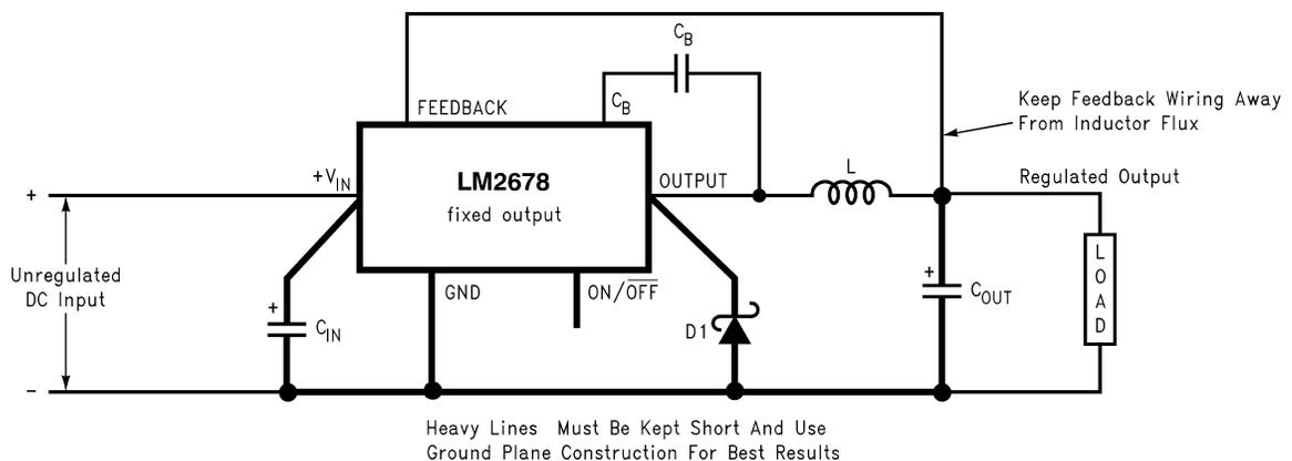
FIGURE 1. Basic circuit for fixed output voltage applications.
