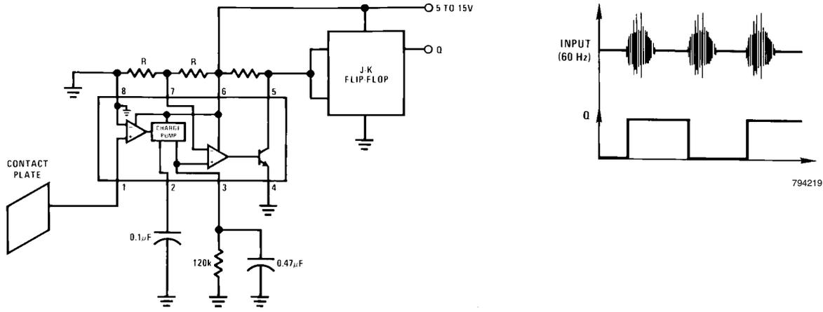
Flashing LED Indicates Overspeed
