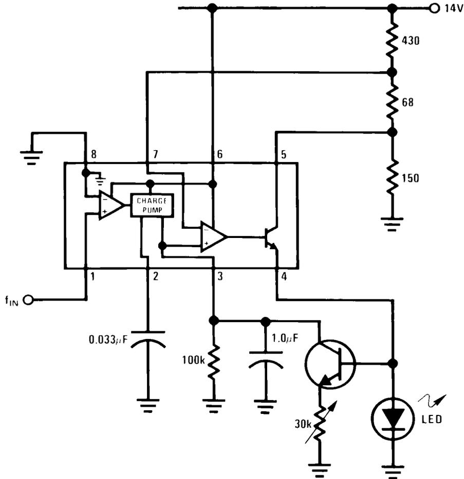
Flashing begins when  $f_{IN} \geq 100$  Hz.
