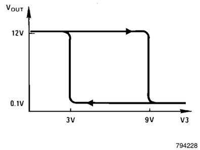
Changing the Output Voltage for an Input Frequency of Zero
