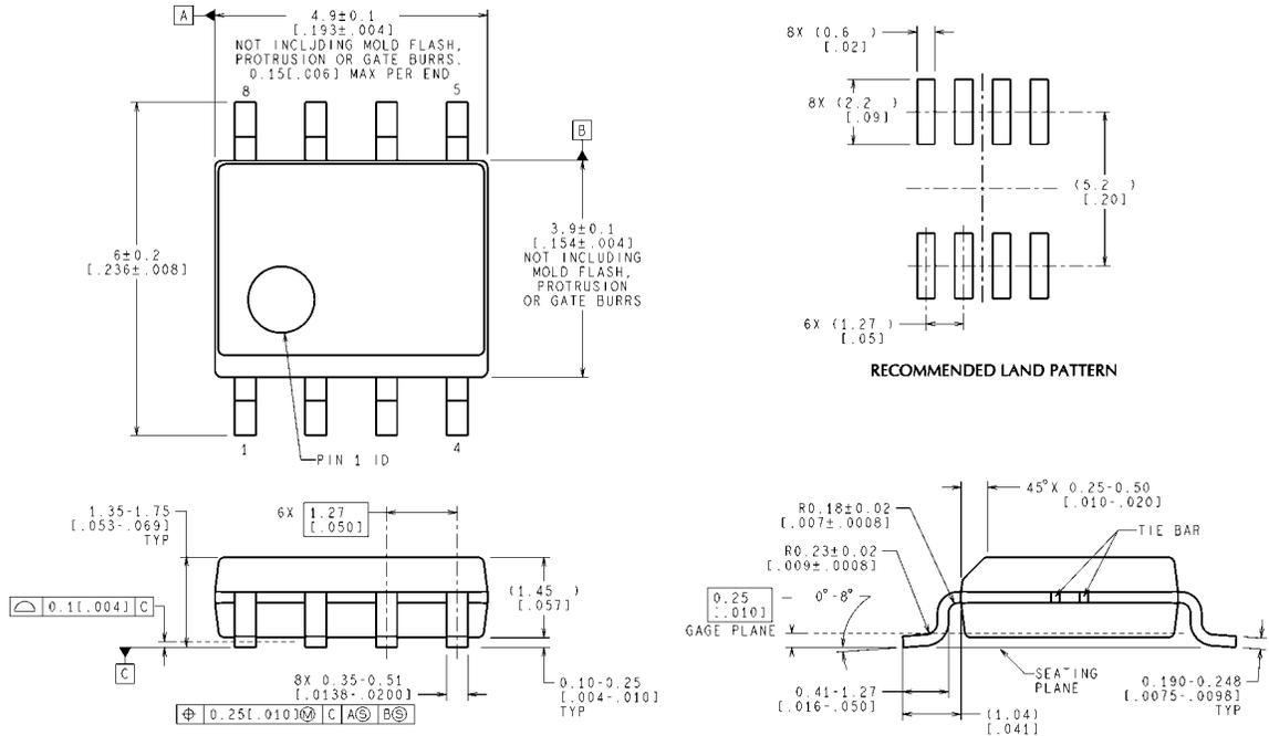
CONTROLLING DIMENSION IS MILLIMETER
