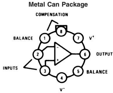
**Note:** Pin 4 connected to case.
