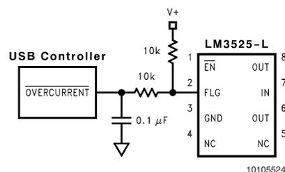
FIGURE 1. Transient Fitter
