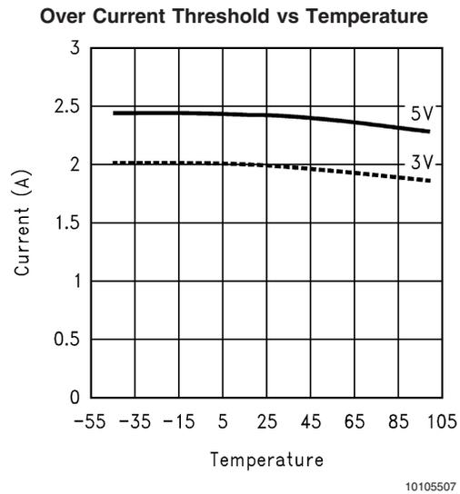
**Typical Performance Characteristics**  $V_{IN} = 5.0V$ ,  $I_L = 500\text{ mA}$ ,  $T_A = 25^\circ\text{C}$  unless otherwise specified. (Continued)
