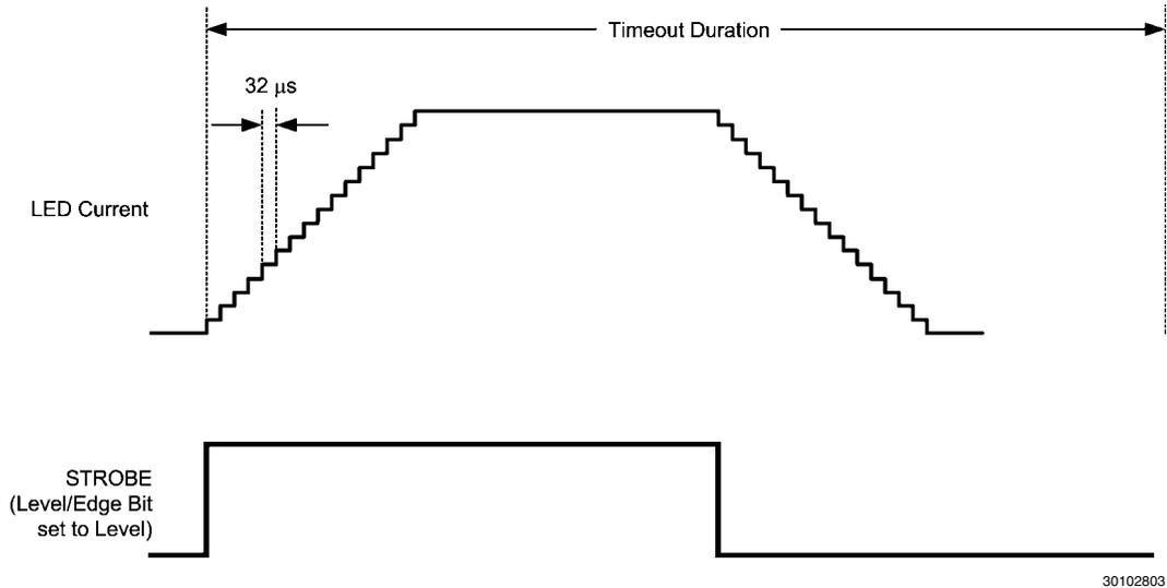
**FIGURE 1. LED Current for STROBE (Level Triggered, Enable Register Bit [5] = 0)
