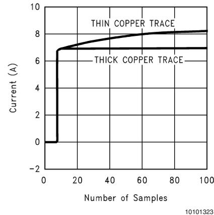
FIGURE 7. Transient Response to 7 Amp Step Current
