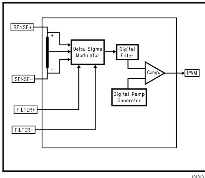
FIGURE 6. Functional block diagram of LM3814 and LM3815
