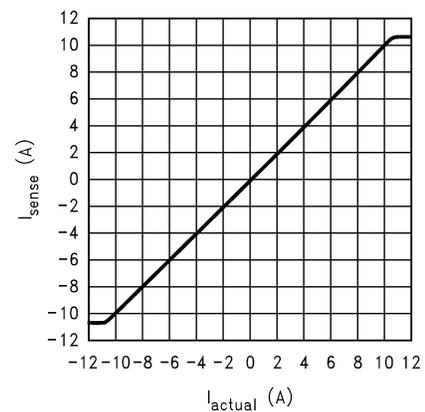
**Typical Performance Characteristics** Supply bypass capacitor is 0.1 $\mu$ F and filter capacitor is 0.1 $\mu$ F. (Continued)
